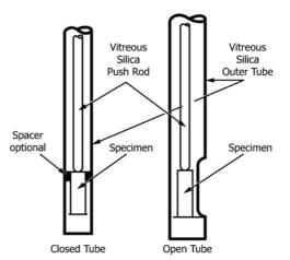
FIG. 1 Common Forms Specimen Holders
