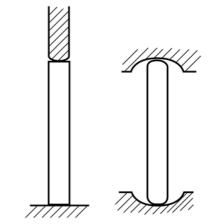
FIG. 2 Suggested Shapes of Specimen's and Push-Rod Ends
